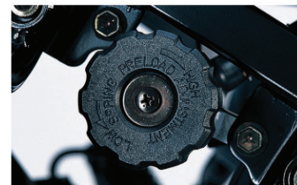
Useful rear spring preload adjustment
